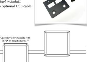
\*\* Modifications required for this mounting configuration: (option #1) Countersink 5mm holes on the opposite side from the 6mm countersinks and use 5x10mm FH screws for PSPD mounting. (option #2) Use longer 6mm FH screws with a spacer so included 5mm Cap Screws clear 80-20 profile. USB cord side exit ONLY.
