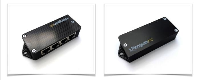
To connect the PSUSB\_28x use the provided cord to connect to any available USB port on your computer. This controller requires no additional software or drivers as it is a standard Windows HID device. The PSUSB\_28x initializes upon being powered up so any setup changes will not take effect until the device is power cycled either by unplugging it or by turning off your computer.
